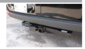
The maximum towing is 3400 kg (7,500 lbs.), the maximum tongue weight is 340 kg (750 lbs.).
